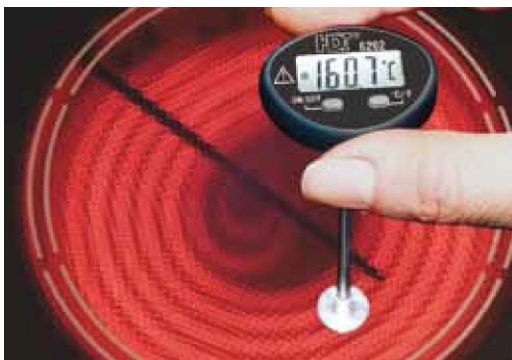
6201 Needle probe -50...+250°C
